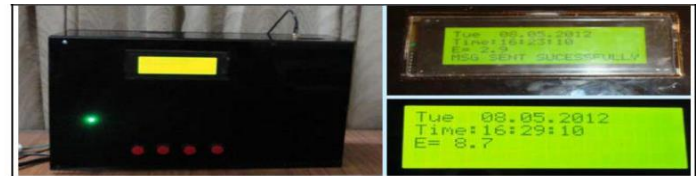
Fig.7 GSM Meter after casing and sample results on display.
